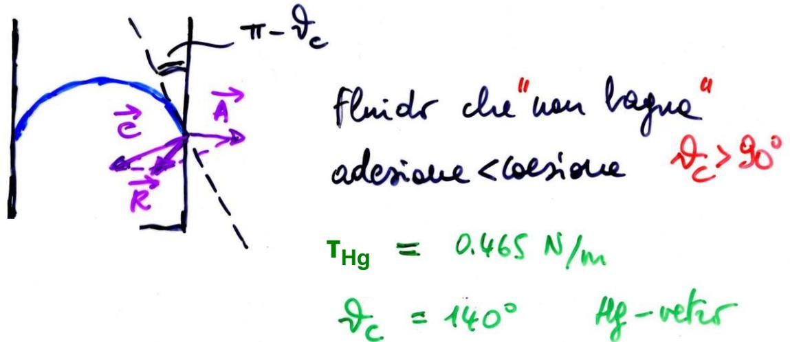
$$T_{\text{Hg}} = 0.465 \text{ N/m}$$
