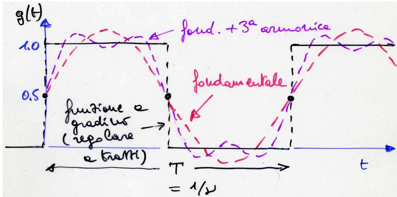
$$f(t) = \frac{1}{2} + \frac{2}{\pi} \left[ \sin\left(2\pi \frac{t}{T}\right) + \frac{1}{3} \sin\left(3 \cdot 2\pi \frac{t}{T}\right) + \dots + \frac{1}{2n+1} \sin\left((2n+1) \cdot 2\pi \frac{t}{T}\right) + \dots \right]$$
