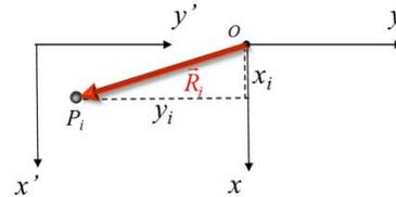
$$\begin{aligned} I_Z &= \sum_{i=1}^n m_i(x_i'^2 + y_i'^2 + a^2 - 2ay_i') \\ &= \sum_{i=1}^n m_i(x_i'^2 + y_i'^2) + \sum_{i=1}^n m_i a^2 - \sum_{i=1}^n m_i(2ay_i') \\ &= I_C + a^2 \sum_{i=1}^n m_i - 2a \sum_{i=1}^n m_i y_i' \end{aligned}$$
